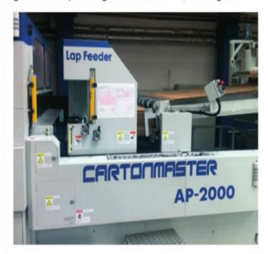
lateral direction, and can be manually adjusted. A gripper bar collects the accurately positioned sheet and transfers it to the die-cutter.
